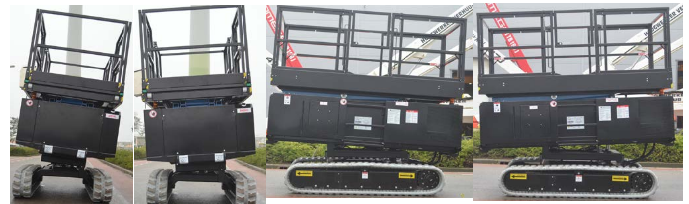
6 degrees Leveling capabilities - fore to aft
